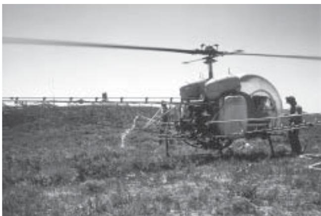
**Figure 40**—Helicopter equipped with a boom sprayer.
