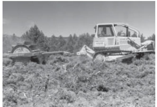
**Figure 35**—Roller chopper being used to kill and cut up pinyon and juniper trees, create a seedbed, and cover seed.
