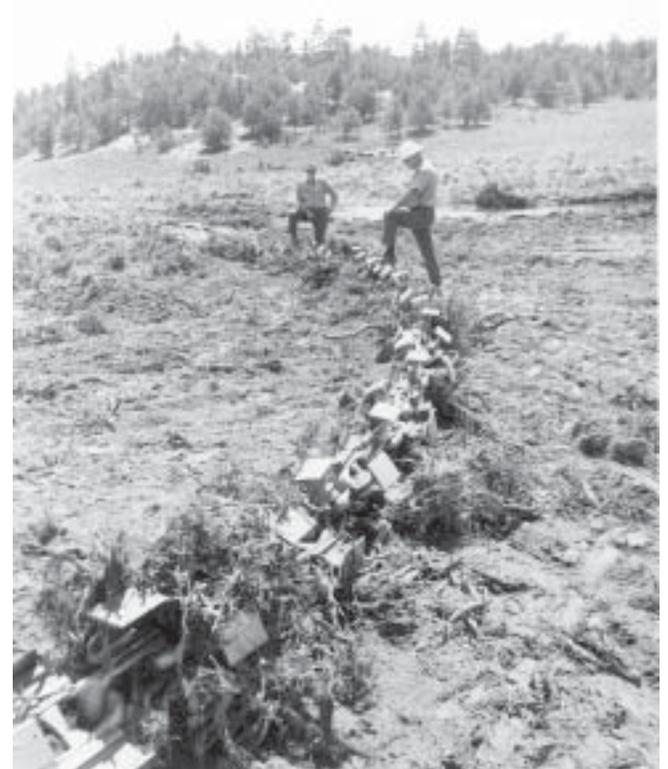
Figure 7—Dixie Sager. Anchor chain with railroad rails welded horizontally to both sides of each link.
