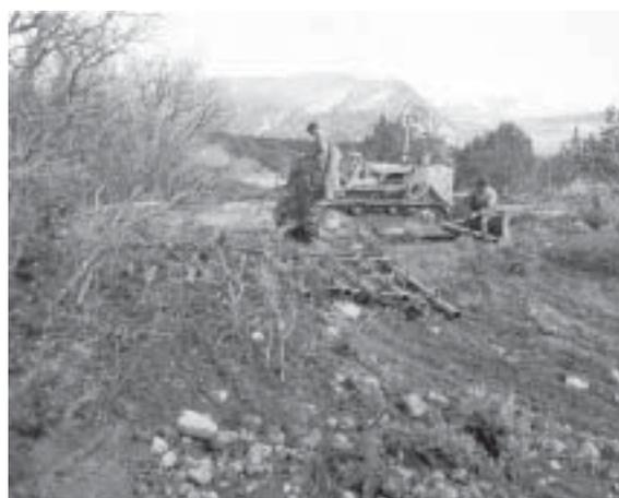
**Figure 11**—Pipe harrow and Hansen seed dribbler being used to seed shrubs and cover herb seeds to improve interspaces between pinyon and juniper trees and Gambel oak. Herbs were broadcast seeded prior to treatment.
