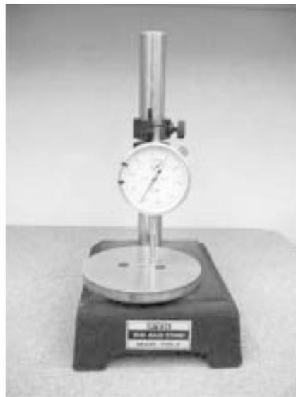
Figure 7.2— Measuring thickness.
