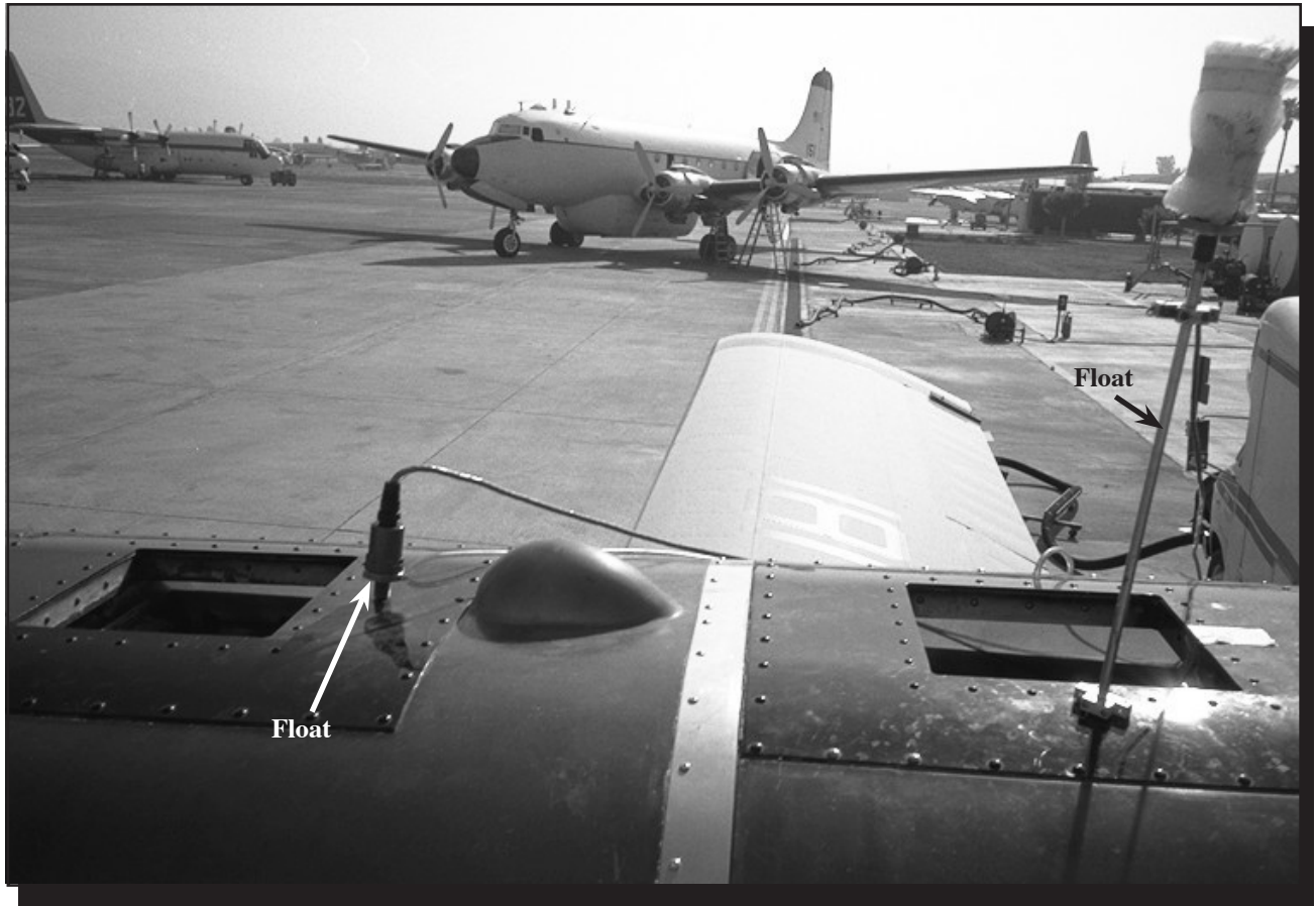
Figure 6—Two floats were mounted in this tank. The float head at the left is nearly flush with the tank cover. Because of the of the tank's vent design, the floats could not be mounted through vent openings.
