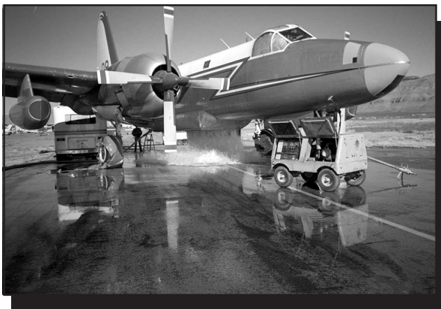
Figure 1—A static test of the Neptune P2V. An auxiliary power unit can supply power, eliminating the need to run the plane's engines during the test.
