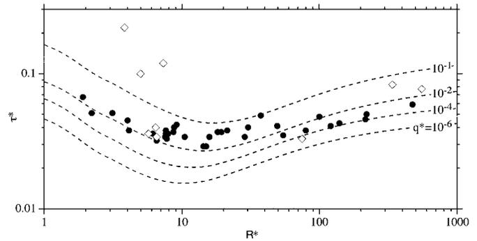
FIG. 7. Dimensionless Shear Stress ( $\tau^*$ ) versus Boundary Reynolds Number ( $R^*$ ) for Data Used by Shields (1936b) (Table 3) (Circles) and for Values Determined from Bed-Load Extrapolation ( $\tau_{c,rm}^*$ , Table 2, Column 7) (Diamonds). Dashed Lines Are Contours of Dimensionless Bed-Load Transport Rate ( $q^*$ ) Predicted from Fig. 7 and Data of Taylor and Vanoni (1972)
