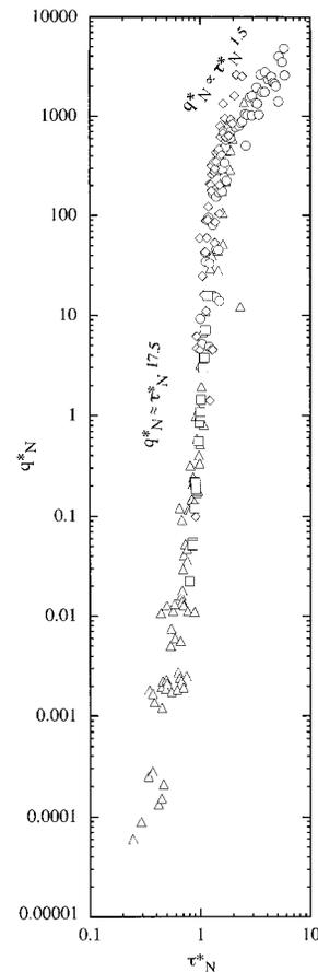
FIG. 8. Normalized Dimensionless Transport Rate ( $q_N^*$ ) versus Normalized Dimensionless Shear Stress ( $\tau_N^*$ ) for Data of Casey (1935a,b) (Diamonds), USWES (1935) (Circles), Paintal (1971) (Triangles), and Taylor and Vanoni (1972) (Squares)
