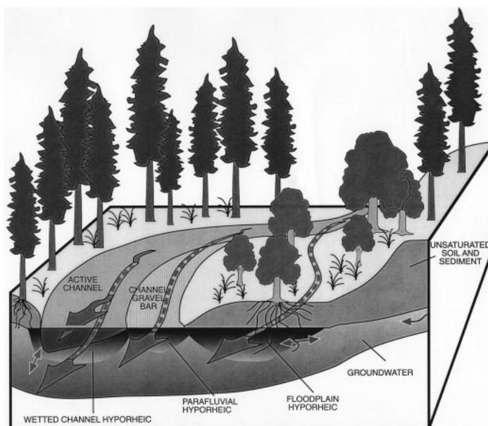
**Figure 11.** Location of three major types of hyporheic zones beneath and adjacent to a river. Single-ended arrows symbolize subsurface flowpaths. Double-ended arrows indicate mixing with adjacent water masses. Although the three zones are shown as distinct regions, in any catchment, they are connected to varying degrees depending on sediment and hydraulic head characteristics.
