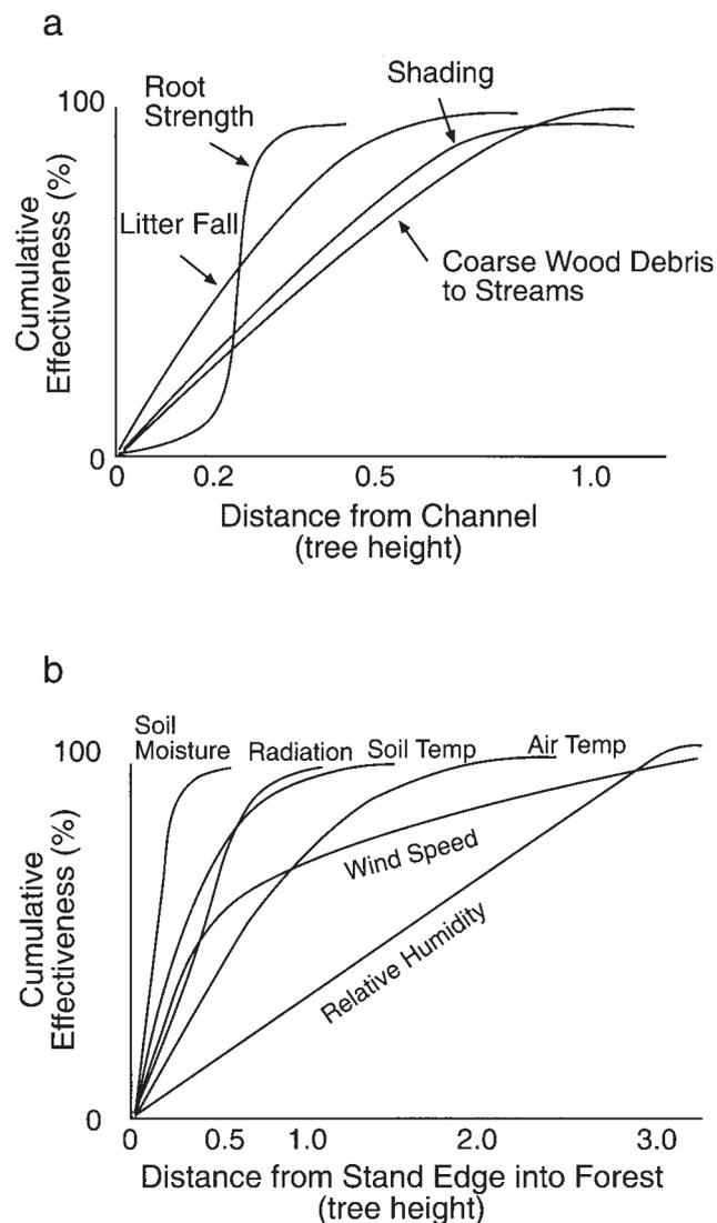
**Figure 10.** The effectiveness of riparian vegetation in supplying ecological services to the river corridor depends on the height of the vegetation and its distance from the stream edge. (a) Cumulative effectiveness of four riparian processes as a function of relative distance from the edge of a stream, in fractions of a dominant tree height. (b) Cumulative effectiveness is shown for six microclimate factors as a function of relative distance from the stream edge. Modified from FEMAT (1993).
