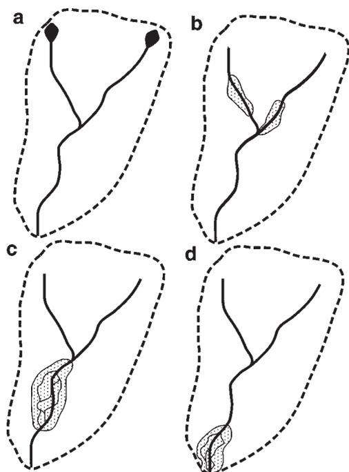
**Figure 6.** Sediment wave propagation through a channel network. Landslides originating at the head of the channel network (a) deliver sediment that rapidly propagates (b) through steep headwater channels to lower-gradient reaches (c) where deposition may trigger channel braiding, which eventually (d) recovers to a single thread morphology. From Montgomery and Buffington (1998).
