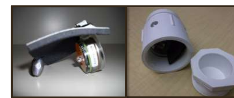
Figure 4. Two potential means for shading a stream sensor from solar radiation: TidbiT with a piece of neoprene zip-tied to the sensor (left) and TidbiT encased in a PVC housing (right).
