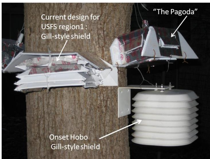
so the measurement device does not heat up. We know that bank thermometers in the summer, your outdoor thermometer etc. are often biased if they are not well shaded. A sensor, placed outdoors that receives direct sunlight will heat above ambient air temperatures, oftentimes by 10 degrees Celcius or more. Housing your sensor in something that blocks incoming radiation, but allows air to flow easily across the sensor is essential to accurately measuring the air
