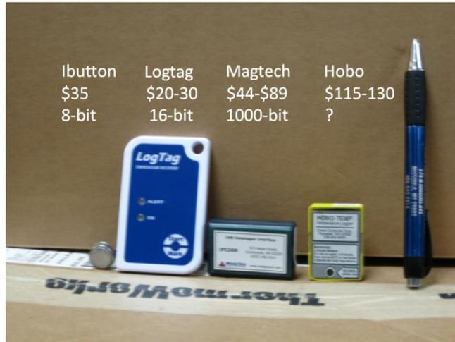
**Thermoworks Logtags** have emerged as a competitor to the iButton. These cost \$30 each (\$19 in bulk) and have nearly the same specifications as iButtons. They are also not waterproof. They have begun custom building these sensors for our USFS monitoring project that have 2x the memory (16,000 measurements). This means we can now sample for a full year at 1 hour interval, or 2.5 years at 90 minute intervals.
