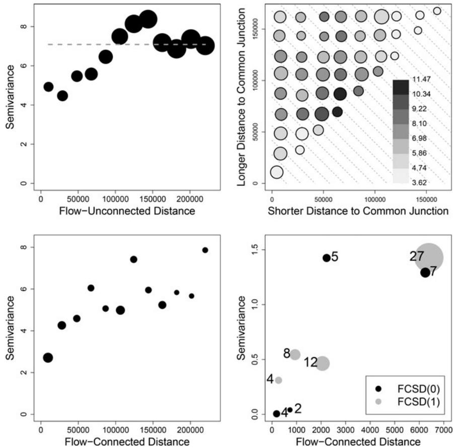
**Figure 6.** Torgegrams for residuals, after removing effects for distance upstream and elevation, of the Lewis and Willamette watersheds stream temperature data. The description is exactly as for Figure 5.
