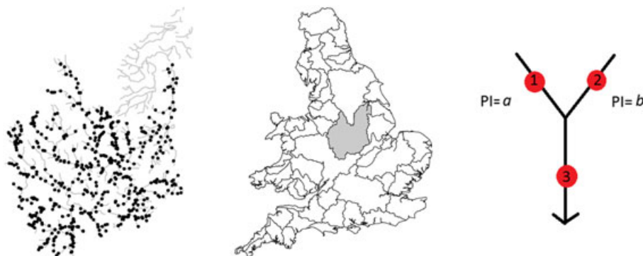
FIGURE 1 River network in Trent catchment area (gray lines) with 566 monitoring sites (black dots), (left). Location of Trent catchment area in England and Wales (middle). Diagram of simple river network with three monitoring sites and corresponding proportional influence (PI) values for upstream segments (right)
