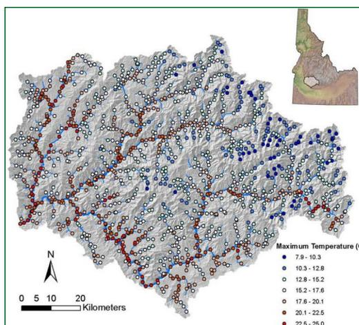
*Predicted maximum summer stream temperatures across the Boise River Basin. This modeling approach uses thermograph data and predictor variables (air temperature, solar radiation, elevation, and stream flow).*
