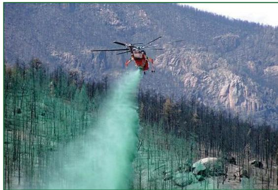
*Aerial application of hydromulch, a matrix of organic fibers mixed with water that binds to the soil surface.*
