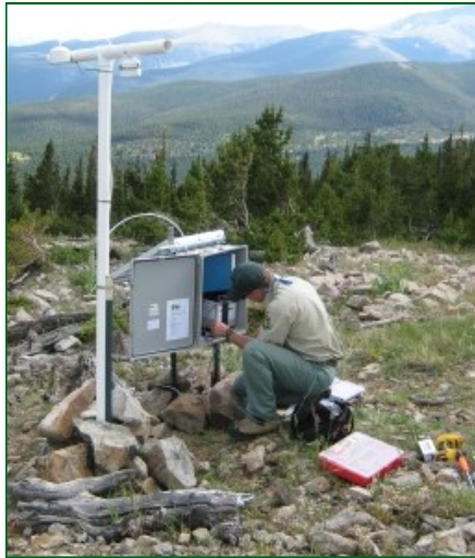
RMRS researchers are using a portable battery powered monitor to evaluate ozone at Trout Creek Pass, Colorado and several other high-elevation locations in the Rocky Mountain West.
