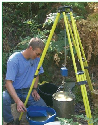
*Measuring sediment using a survey tripod.*
