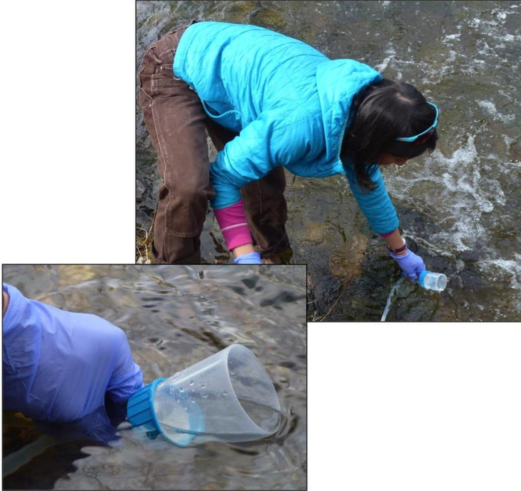
**Figure 4.** Collecting the field sample in a large stream. Cup should be placed far enough into the current to ensure that only upstream water enters the cup.
