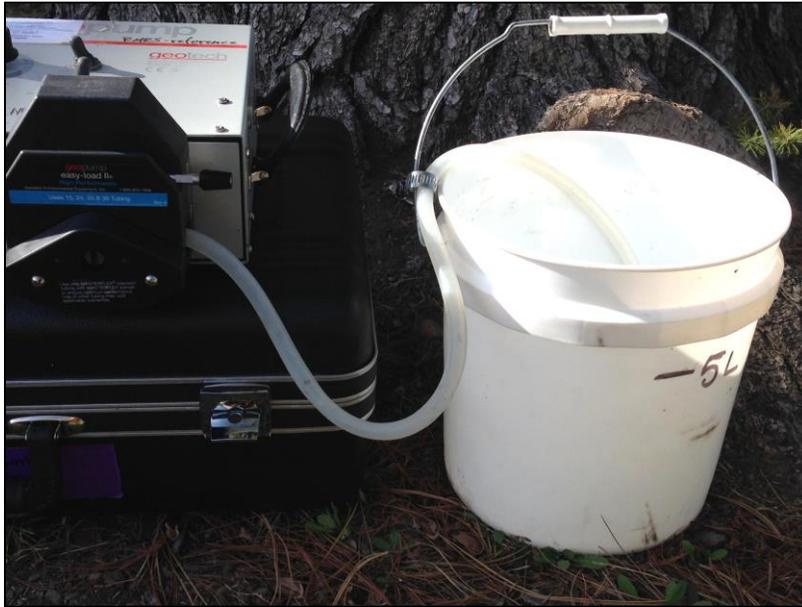
**Figure 2.** Outflow end of hose threaded through hose clamp and placed into outflow bucket
