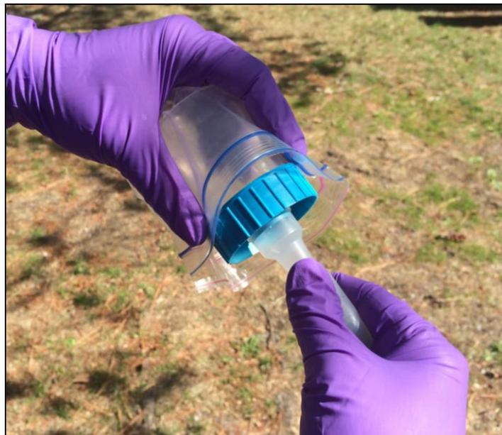
**Figure 3.** Attaching filter holder adaptor and using packaging bag to handle hose
