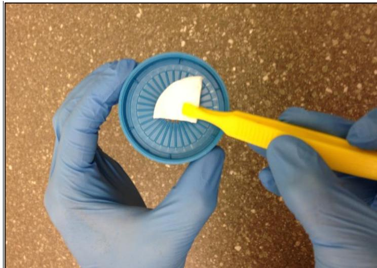
**Figure 6.** Folding the filter paper, filtering side in
