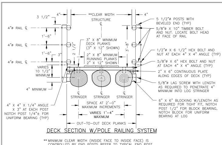
CONTROLLED BY END POSTS REFER TO TYPICAL END POST CONNECTION DETAILS ON THIS SHEET.
