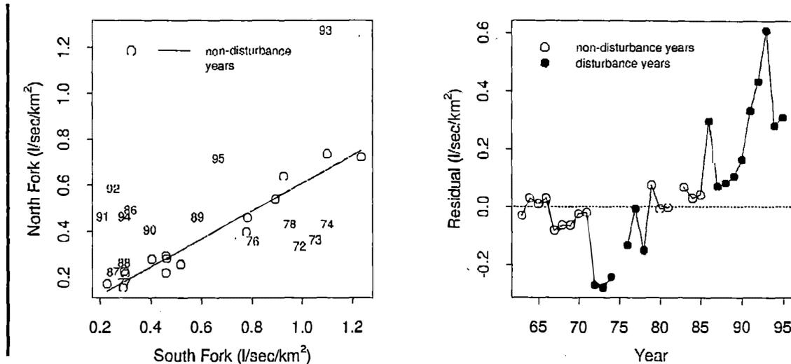
**Figure 1.** Relation between minimum summer streamflow in the North and South Forks of Caspar Creek, 1963-1995, the regression line is based on non-disturbance years; and residuals of observed streamflow from the non-disturbance regression.
