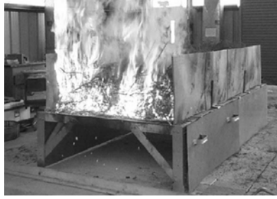
Fig. 1. Fuel bed constructed of live foliage and branches of chamise with 2.0 m long, 1.0 m wide and 0.4 m depth. The fire illustrates the initial ignition.
