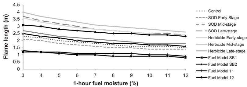
Fig. 4. Comparison of predicted flame length to existing and custom fuel models by condition/time category.
