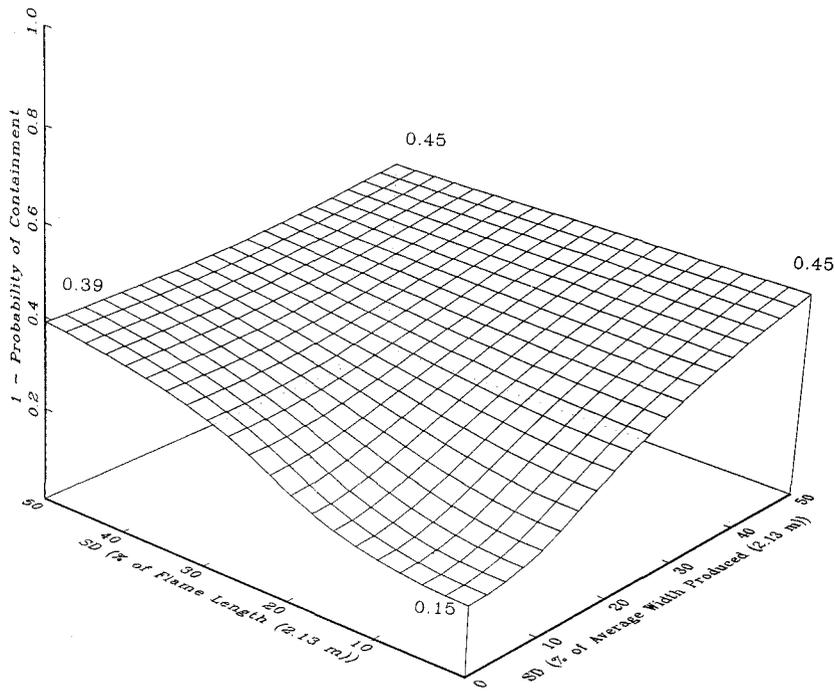
Figure 5. Plotted is (1.0 -Probability of containment) for a 2.13 meters expected flame length and 2.13 meters expected width produced. The standard deviations are expressed as a percentage of the expected flame length and width produced.
