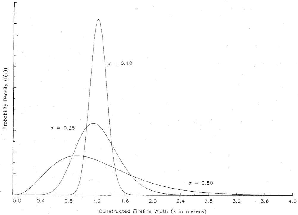
**Figure 2(b).** The probability density function for the construction of an expected fireline width of 1.22 meters and 3 standard deviations ( $\sigma = .1 \cdot 1.22, .25 \cdot 1.22,$  and  $.5 \cdot 1.22$  meters). The ordinate is scaled so that the area under the curve is equal to one.
