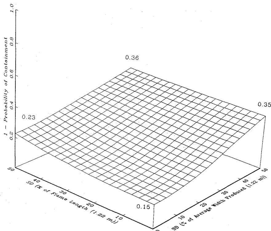
Figure 3. Plotted is (1.0 - Probability of containment) for a 1.22 meters expected flame length and 1.22 meters expected width produced. The standard deviations are expressed as a percentage of the expected flame length and width produced.
