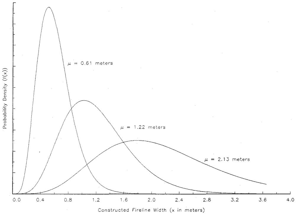
**Figure 2(a).** The probability density function for the construction of fireline width for 3 expected widths ( $\mu$ ) and standard deviation equals 40% of the expected width. The ordinate is scaled so that the area under the curve is equal to one.
