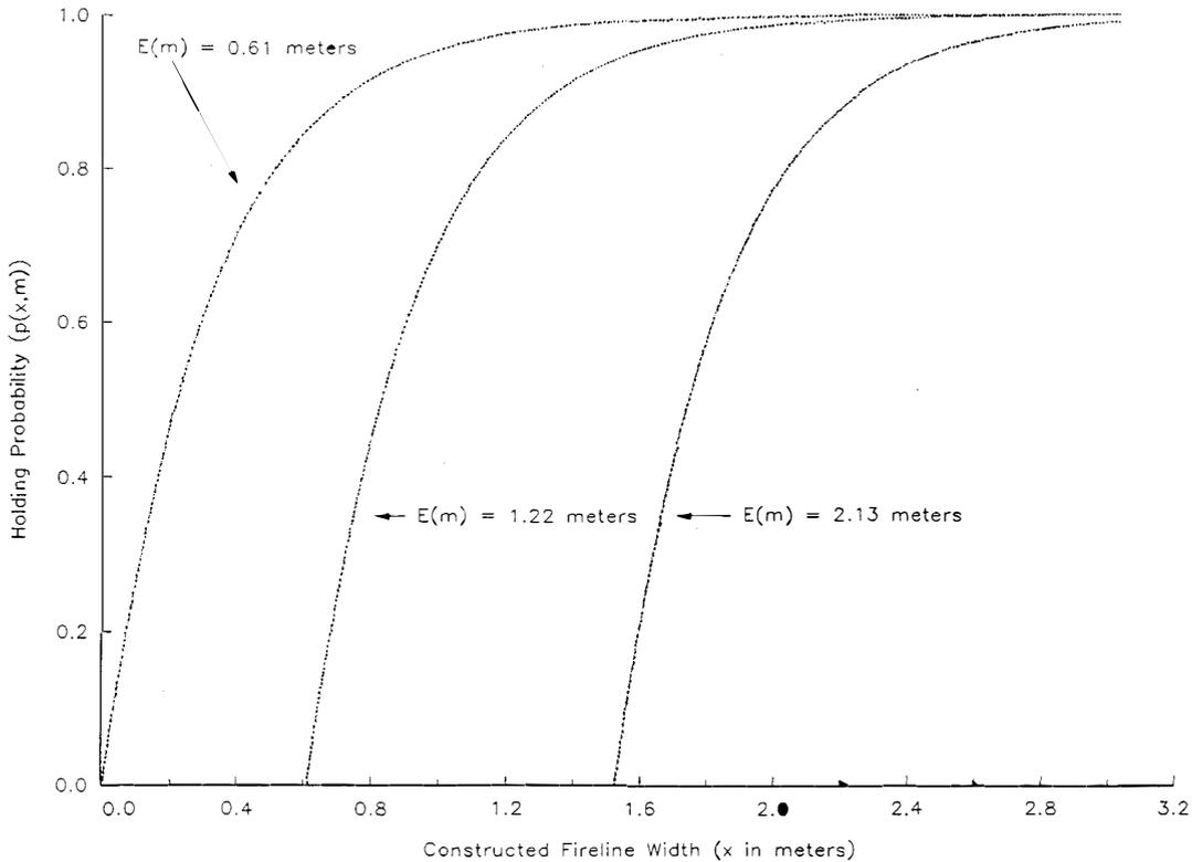
**Figure 1.** Plotted are the probability of holding ( $p(x,m)$ ) for average flame lengths of .61, 1.22, and 2.13 meters as a function of the fireline width constructed ( $x$ ).
