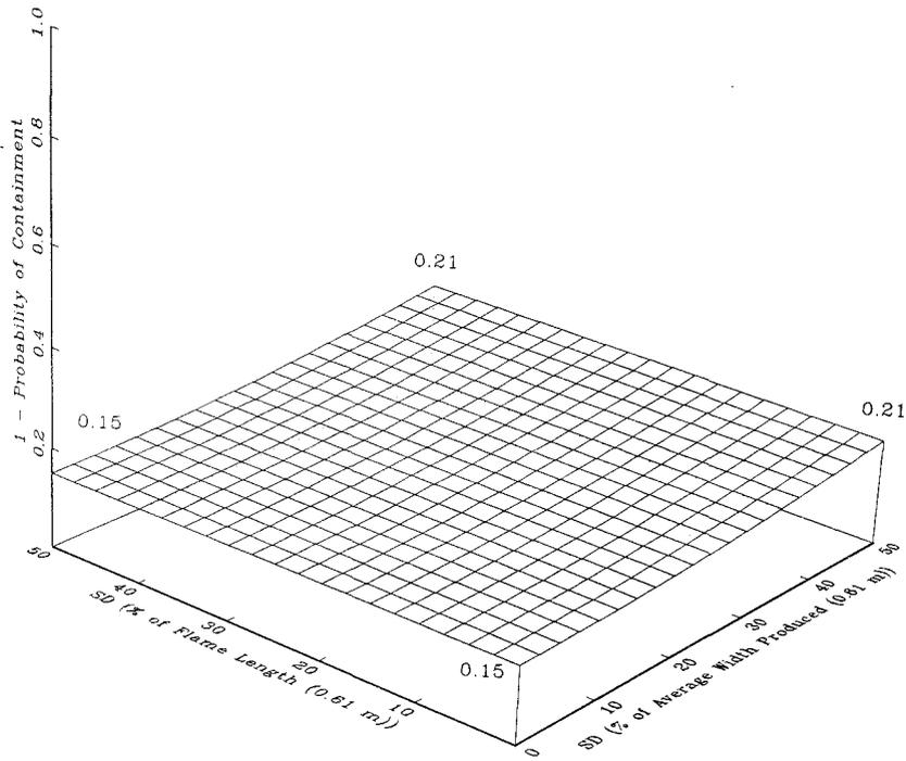
Figure 4. Plotted is (1.0-Probability of containment) for a .61 meters expected flame length and .61 meters expected width produced. The standard deviations are expressed as a percentage of the expected flame length and fireline width produced.
