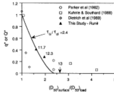
Fig. 6. Plot of  $q_*$  or  $Q_*$  versus degree of armoring,  $(D_{50})_{sur}/(D_{50})_{load}$ . The scatter of points about the decreasing trend of  $q_*$  with  $(D_{50})_{sur}/(D_{50})_{load}$  is due to variations in  $\tau_G/\tau_{cl}$ . The plot of  $\tau_G/\tau_{cl} = 2.4$  describes the mean trend of our experiment.
