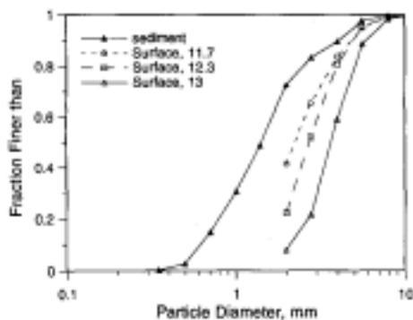
Fig. 1. Particle size distributions of sediment that was filled and fed into the flume and of the bed surface at the ends of runs 11.7, 12.3, and 13.
