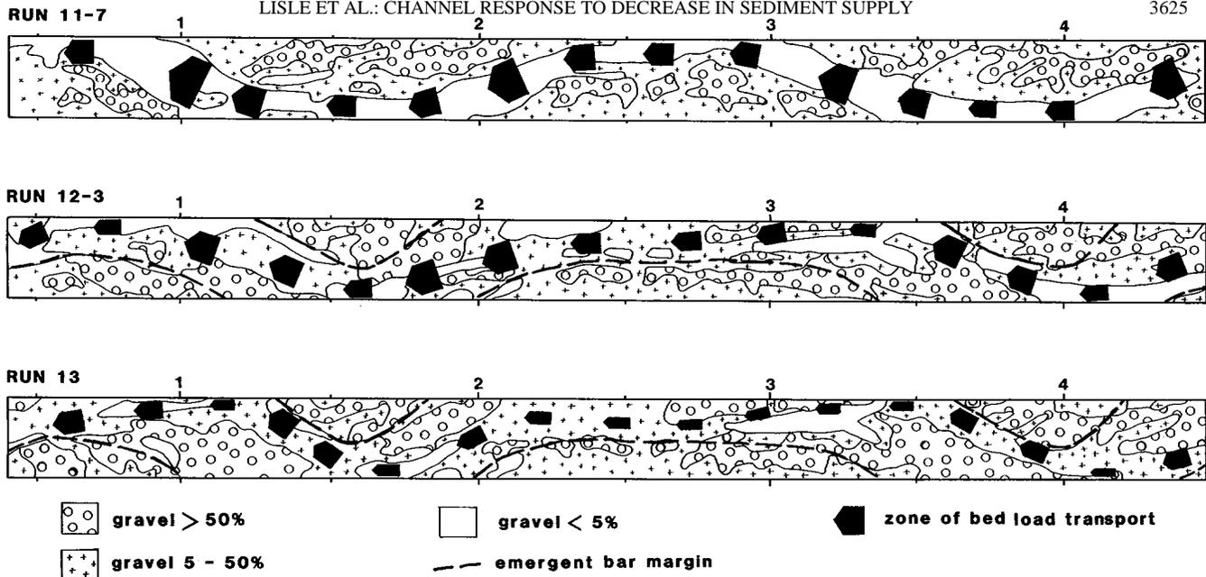
Fig. 3. Bed load corridor and bed surface facies, runs 11.7, 12.3, and 13.
