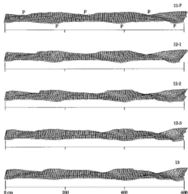
Fig. 4. Oblique view of the lower 6 m of channel at the end of runs 11.7, 12.1, 12.2, 12.3, and 13. Flow is from right to left. There is no vertical exaggeration. The locations of pool deeps are denoted by *p* in run 11.7; they shift upstream in subsequent runs.
