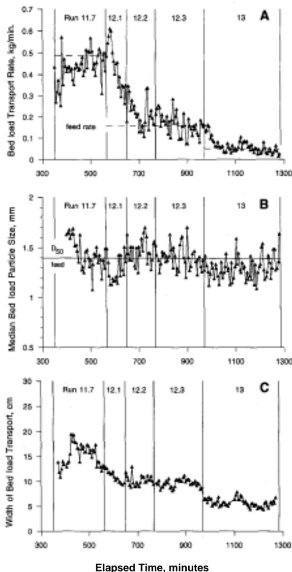
Fig. 2. Variations with elapsed time of (a) bed load transport rate at the flume outlet; (b) median particle diameter of bed load; and (c) width of the corridor of intense bed load transport. Figures 2a and 2b are reproduced from Iseya *et al.* [1989].
