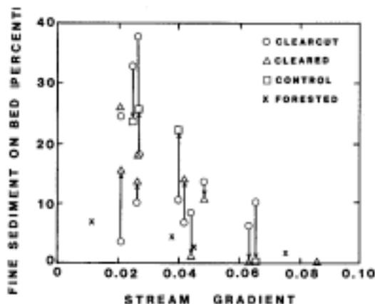
FIGURE 6.-Percentage of the bed surface covered by fine sediment (<4 mm diameter) in relation to stream gradient for eight streams on Prince of Wales Island, Alaska. Arrows show the chronological order of data points for individual reaches; circles represent clear-cut reaches in 1978, before treatment.
