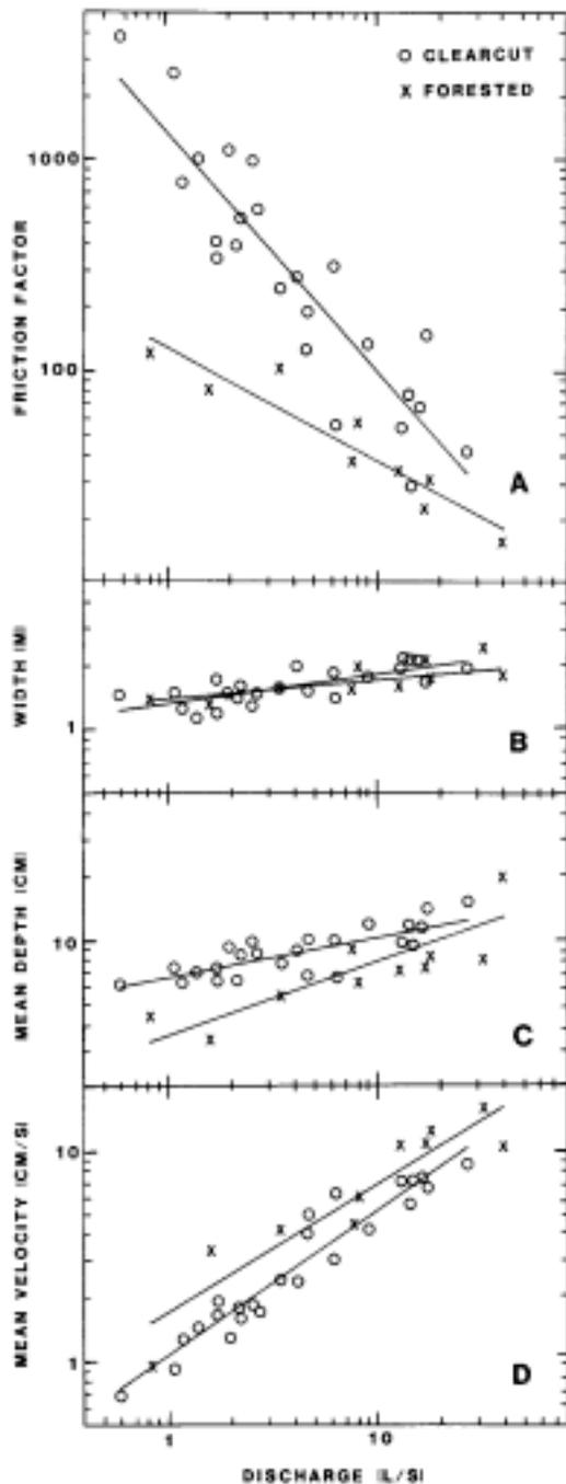
FIGURE 3.- Relationships of water velocity, stream depth and width, and friction factor to stream discharge for four forested reaches and 13 clear-cut reaches of eight streams on Prince of Wales Island, Alaska.
