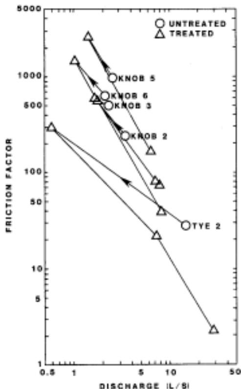
FIGURE 4.- Effects of debris removal on the friction factor in Knob and Tye creeks on Prince of Wales Island, Alaska, in relation to discharge 1978-1981. Arrows show the chronological order of data points for individual reaches; circles represent 1978, before treatment.
