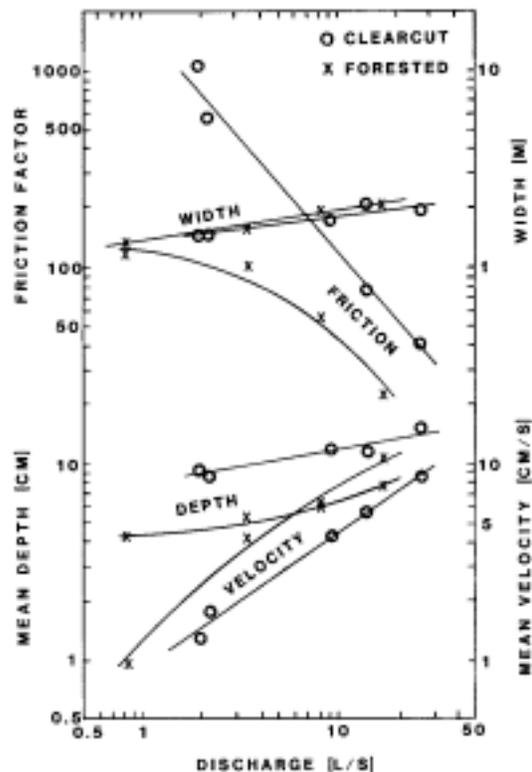
FIGURE 2.- Relationships of water velocity, stream depth and width, and friction factor to stream discharge for a forested reach (Three-Tenths Mile Creek) and an untreated clear-cut reach (Knob Creek, reach 1), Prince of Wales Island, Alaska.
