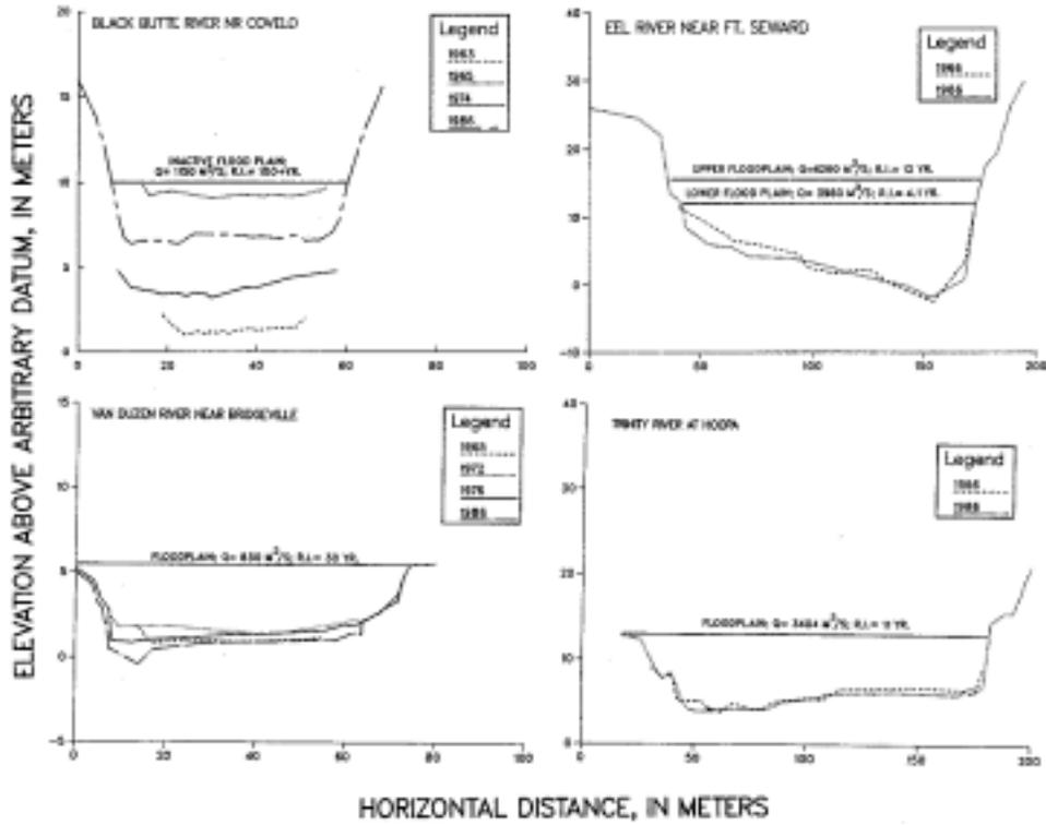
Figure 2. Channel cross sections at study sites. Water discharges (Q) and recurrence intervals of those discharges (R.I.) are shown on lines representing major floodplain levels. The inactive floodplains of the Black Butte River and the upper floodplain of the Eel River are located upstream of those sites.
