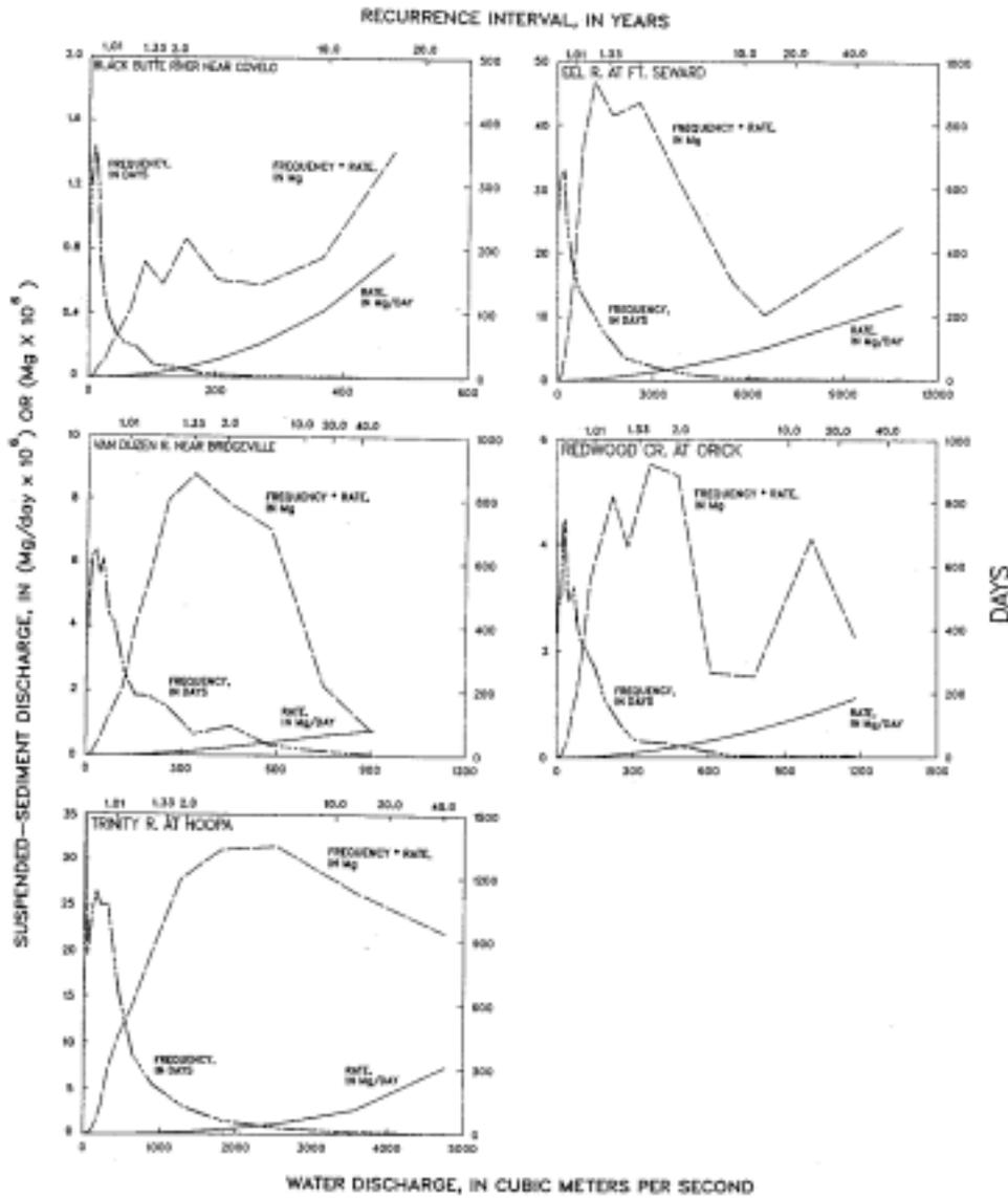
Figure 3. Graphs showing sediment transport rate (in Mg/day), frequency of occurrence of water discharge (in days), and the product of frequency of occurrence and sediment transport rate (in Mg) at study sites.
