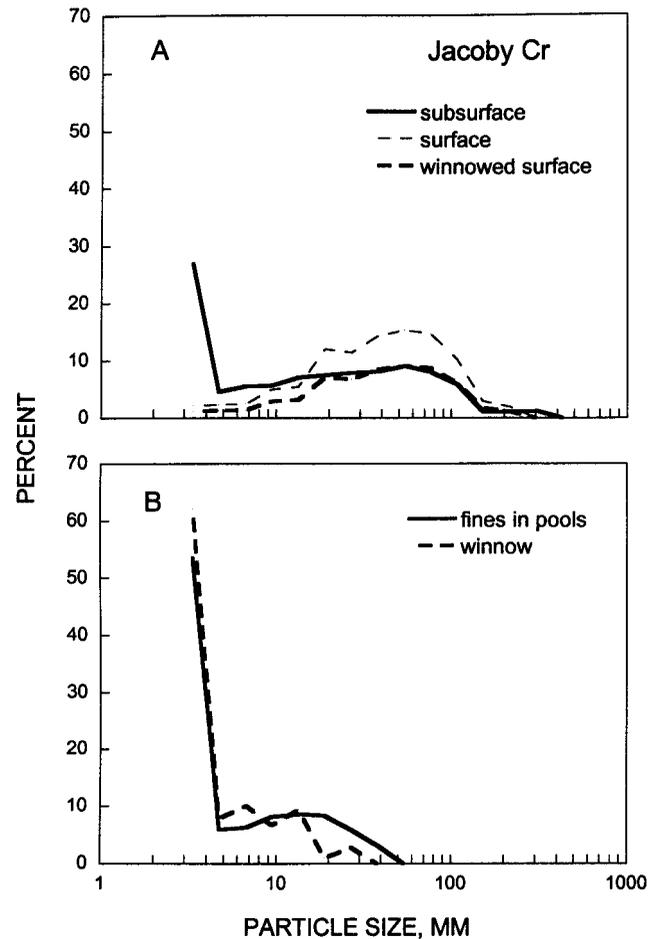
**Figure 5.** Particle size distributions of fine bed material from pools and matrix material estimated from surface and subsurface size distributions for Jacoby Creek, illustrating a “good fit.” The finest size range is for particles  $<4$  mm. (a) Subsurface, surface, and winnowed surface. The matrix is calculated by subtracting the winnowed surface from the subsurface. (b) Fine bed material in pools and estimated matrix.
