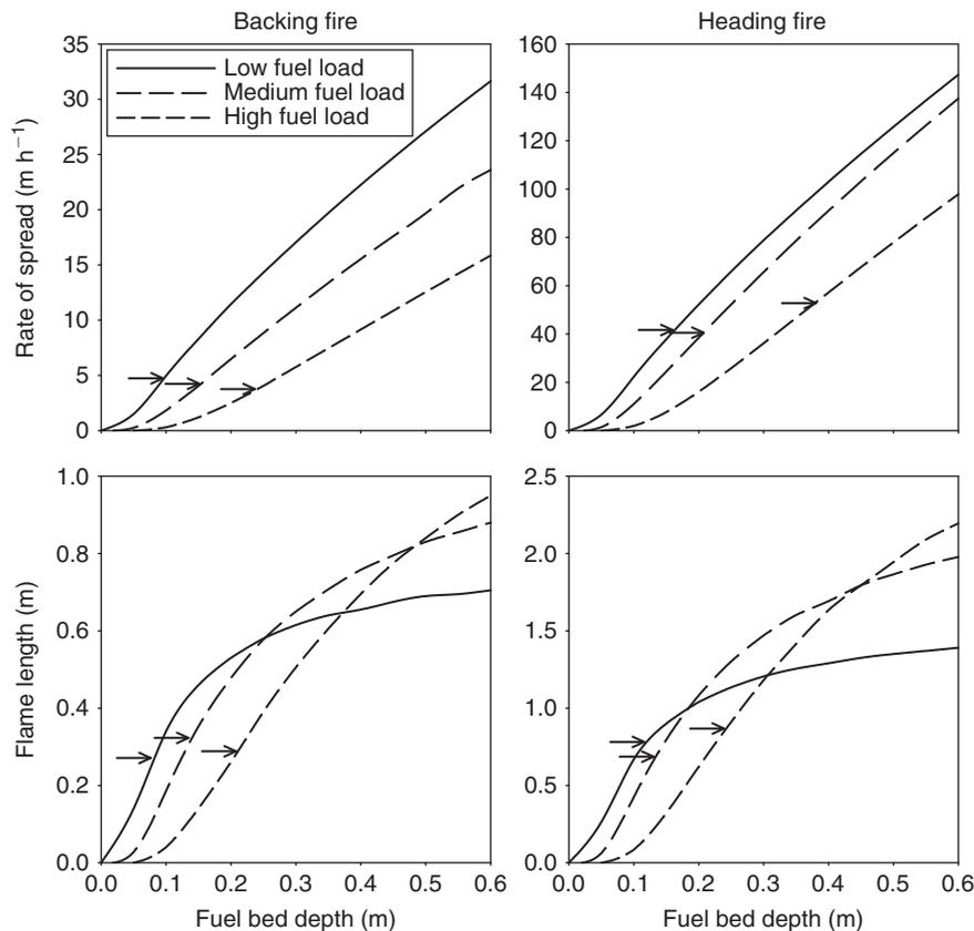
**Fig. 2.** Predicted rates of spread and flame lengths for backing fire and heading fire when depth of the fuelbed is varied. Fire behaviour outputs were modelled with BehavePlus5.0, using custom fuel model inputs (with the exception of fuelbed depth) given in Table 2. Arrows show the actual rates of spread and flame lengths for prescribed burns at Challenge and Whitmore.
