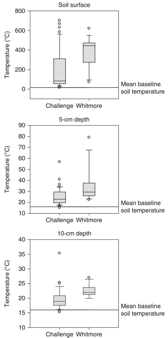
Fig. 4. Maximum temperature reached at the duff-mineral soil boundary, 5 and 10-cm soil depths at Challenge and Whitmore, measured using 12 thermocouples deployed per layer per site. Lines within box plots (25th to 75th percentile) show the median, with whiskers indicating the 10th and 90th percentiles. Outliers are shown as circles.
