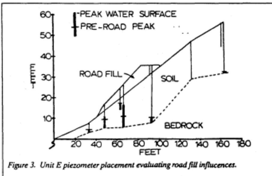
Figure 3. Unit E piezometer placement evaluating road fill influences.
