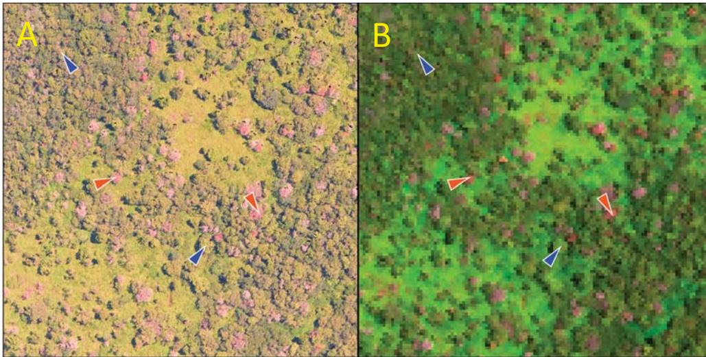
**Figure 2.** Example images from the Carnegie Airborne Observatory: (A) high-resolution digital color camera and (B) visible-to-shortwave infrared (VSWIR) imaging spectrometer showing suspected ROD-infected brown-state crowns and green crowns. Red arrows point to representative brown-state trees and blue arrows point to healthy green trees.
