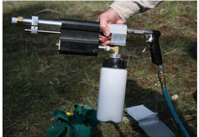
**Figure 1.** PODDS used to spray flakes on individual lodgepole tree boles.
