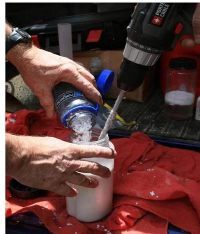
**Figure 2.** Mixing verbenone flakes with sticker and thickener in 1000-ml bottle.
