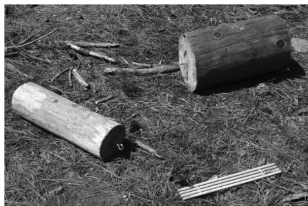
Fig. 2. One set of fuel sticks (10-h) and two size classes of large-diameter fuels (1000- and 10 000-h) were arranged randomly at each of 12 fuel-moisture stations per unit.
