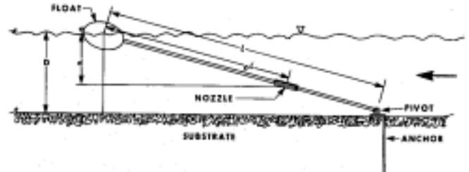
Figure 2. Intake Boom and Mounting Mechanism.
