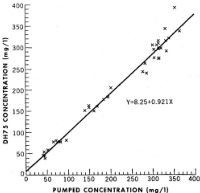
Figure 3. Simultaneous Concentrations of Pumped and Depth Integrated Hand Samples of Janes Creek, Near Arcata, California.
