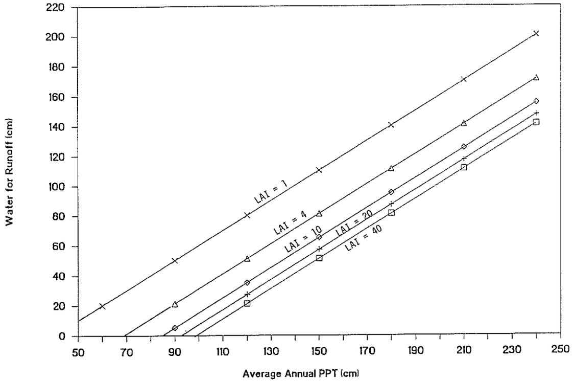
Figure 3—The WRENSS version of PROSPER estimates annually available water for runoff as a function of average annual precipitation (PPT) and leaf area index (LAI).
