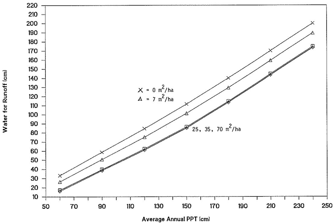
Figure 4—The WRENSS version of the snow model WATBAL estimates annually available water for runoff as a function of average annual precipitation (PPT) and basal area. Estimates are presented for the south energy aspect.
