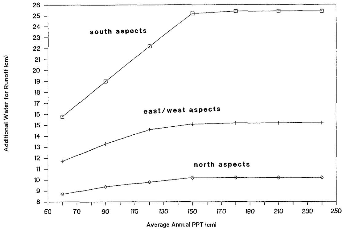
**Figure 8**—Estimated changes in annual runoff with 100 percent basal area reduction can be calculated as a function of annual precipitation and energy aspect in snow-dominated hydrologic regimes.
