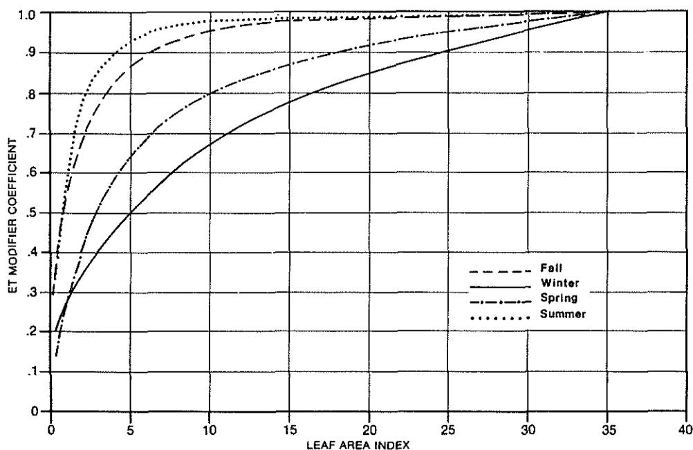
Figure 2—The WRENSS version of PROSPER uses coefficients to modify evapotranspiration (ET) on the basis of leaf area index (LAI) and season.
