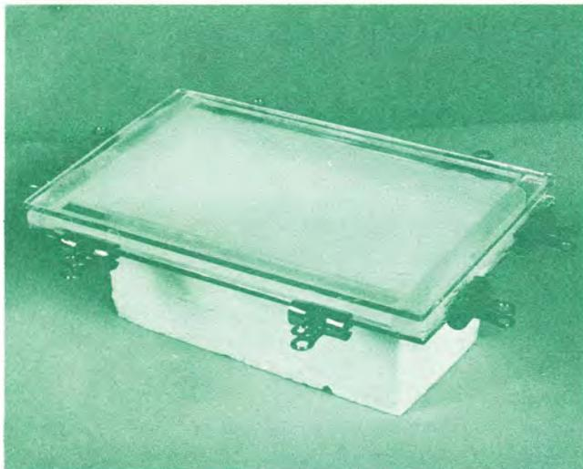
**Figure 1**—Mold with starch gel in place. Top and bottom pieces are of plate glass, separated by plastic spacers on all four sides. Clips hold the spacers in place. After the gel is poured, the top plate is laid over it.
