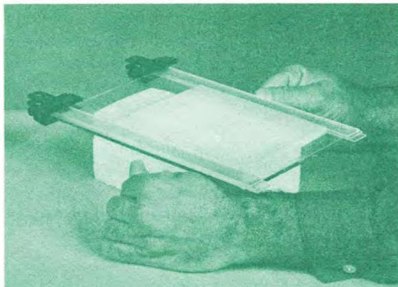
**Figure 5**—Gel being sliced before staining. A piece of fishing line is used as a cutter to produce five layers.
