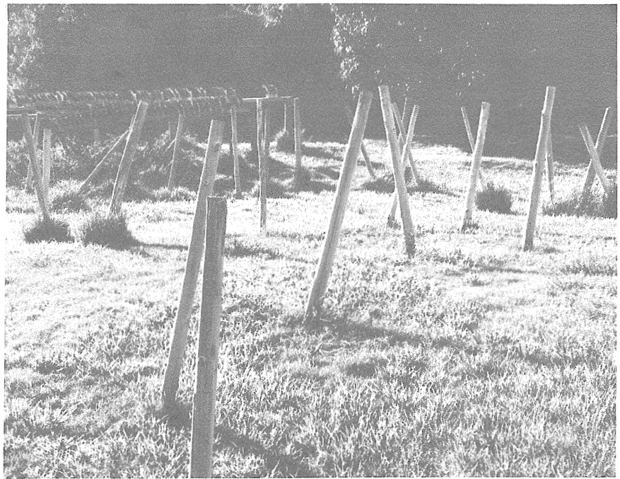
Round posts of 10 Hawaii-grown species were set up in Makiki Valley, Honolulu, in 1961, top. Some posts had been treated with copper chromate-copper arsenate by the double-diffusion process. After 10 years, bottom, only a few posts remain. The missing posts broke off at ground level from decay or termite attacks, and were removed. Another wood durability test underway is shown in the background.
