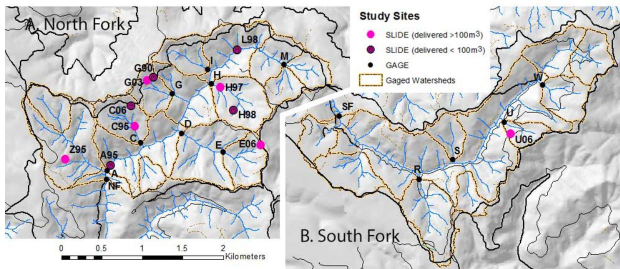
Figure 1—Post-1985 landslides of >100 m<sup>3</sup> in the A. North and B. South Fork Caspar Creek Watersheds. Single and double letters—initials of the gage names—indicate locations of the gages analyzed.
