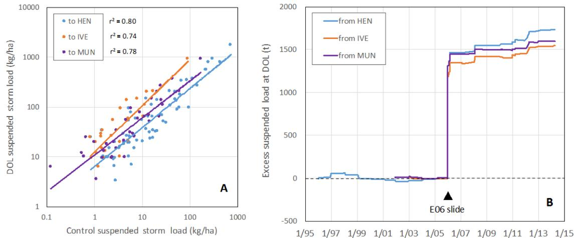
Figure 2—A. Pre-slide relations between storm suspended sediment loads at DOL and at controls HEN, IVE, and MUN; and B. cumulative excess suspended sediment at DOL between 1/1/1995 and 8/1/2014.
