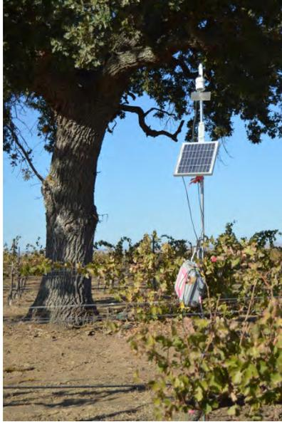
Figure 1—Echolocation recording system clamped to a vine post at one of our tree sites. The photograph shows an Anabat II detector echolocation microphone with a polycarbonate sound reflector plate mounted at the top of a 3-m conduit, a 10 watt solar panel that charges a 9-volt battery housed with an Anabat recorder and Z-CAIM (see text) in the weather proof and dust proof container. (Photo: S. Giordano)
