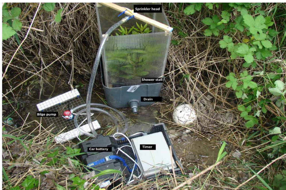
Figure 2—“Shower” apparatus for exposing plants to Phytophthora ramorum inoculum in stream water. Potted rhododendron plants were placed inside the shower and overhead irrigated with water, which was pumped from the stream at three 1-minute intervals programmed into the timer. Plants were exposed for 1 week, after which time they were taken to the biocontainment facility at Washington State University-Puyallup for incubation.
