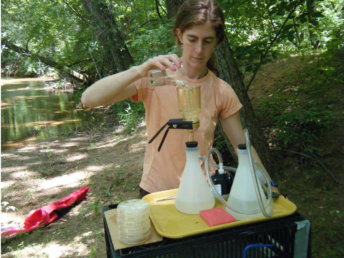
Figure 2—Each month, all water sub-samples were processed at the stream site to maintain sample integrity and prevent potential propagule degradation during storage and transit.
