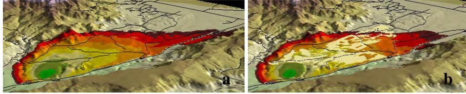
**Figure—2** Eight-hr FARSITE simulation for the 85<sup>th</sup> percentile weather and fuel condition, pre-treatment (a) and post-treatment (b). Each color represents a 1 hr progression of the fire overlaid with roads (black) and the treated landscape (light yellow). Black Ridge is in the foreground and the Pine Valley Mountains in the background (NW). Fuel modifications reduced the size of the fire by approximately 1,500 ac (18 percent).
