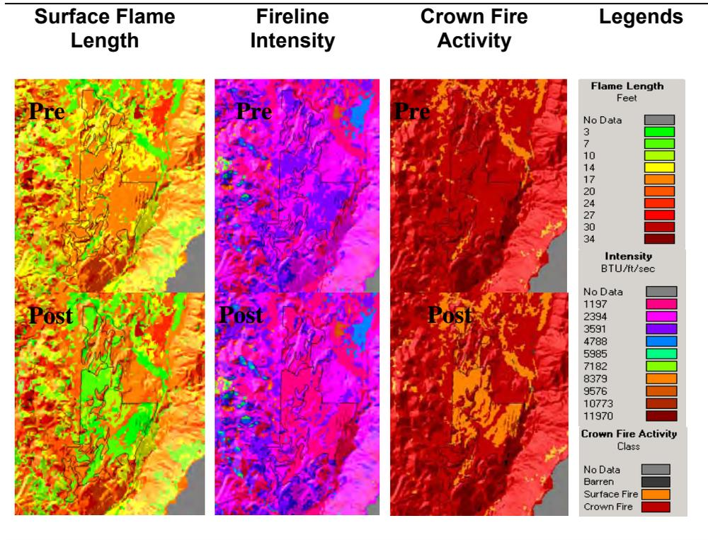
**Figure 3**—FlamMap output for the 85<sup>th</sup> percentile condition, pre-treatment (top) and post-treatment (bottom). The project area boundary is overlaid in black and runs north to south—about 4.5 miles.
