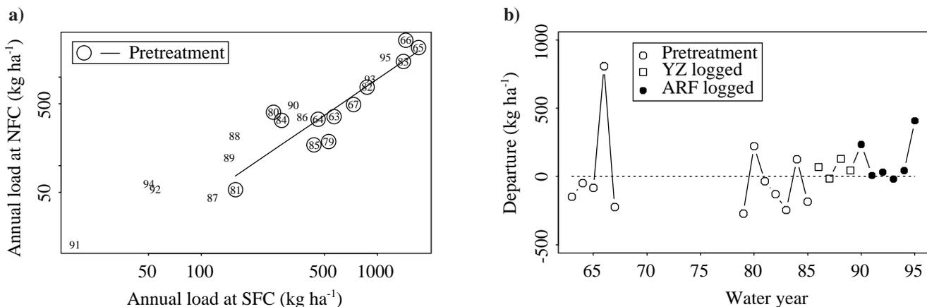
**Figure 3**—(a) Relation between estimated annual suspended sediment loads at North Fork Caspar Creek (NFC) and South Fork Caspar Creek (SFC) from 1963 to 1967 and 1979 to 1995, excluding years when sediment was elevated following logging in the South Fork. Pretreatment regression line is fit to the water years before roading and logging activity in the North Fork. (b) Time series of departures from the regression line.
