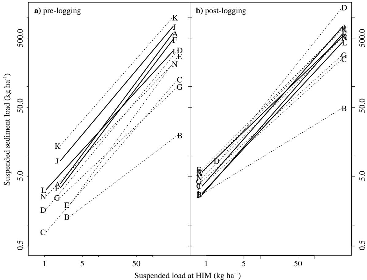
**Figure 10**—Regression lines for storm suspended sediment loads at treated watersheds in the North Fork, predicted from HIM control (mean suspended load of unlogged tributaries HEN, IVE, and MUN). (a) pre-logging, and (b) post-logging. Solid lines represent main-stem stations and dashed lines represent tributary stations.
