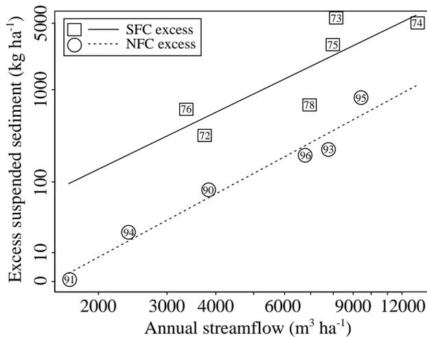
**Figure 11**—Relations between annual excess suspended sediment and annual streamflow for six years after logging in the South Fork and North Fork. South Fork excess loads are the departures from the pretreatment regression of figure 2. North Fork excess loads are the sums of storm departures from the pretreatment regression of figure 6.
