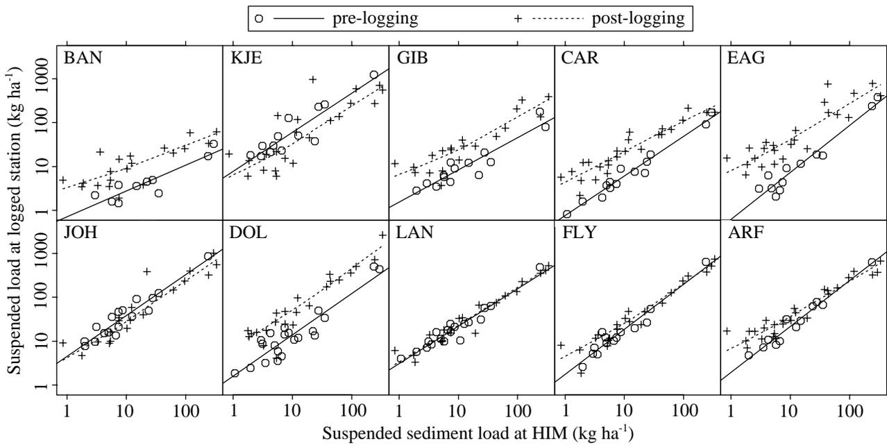
**Figure 7**—Relations between storm suspended sediment loads at logged subwatersheds in the North Fork and HIM control (mean suspended load of unlogged tributaries HEN, IVE, and MUN) from 1986 to 1995. Pre-logging regression lines are based on pretreatment years that are specific to each subwatershed. Post-logging relations are not assumed to be linear, hence were fitted by locally weighted regression (Cleveland 1993).
