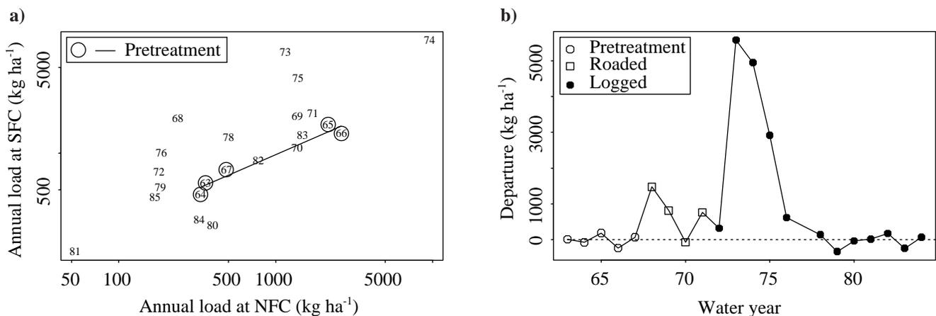
**Figure 2**—(a) Relation between estimated annual suspended sediment loads at South Fork Caspar Creek (SFC) and North Fork Caspar Creek (NFC) from 1963 to 1985. Pretreatment regression line is fit to the water years before roading and logging activity in the South Fork. (b) Time series of departures from the regression line.
