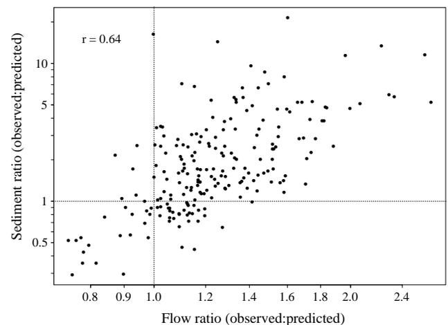
**Figure 8**—Relation between post-logging ratios of observed to predicted storm flow and suspended sediment load for all North Fork subwatersheds. Predictions are for undisturbed watersheds based on aggregated regression models using HI control (mean response of unlogged tributaries HEN and IVE).
