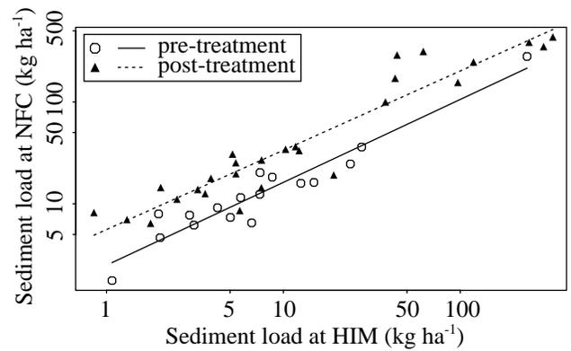
**Figure 6**—Relation between storm suspended sediment loads at North Fork Caspar Creek (NFC) and HIM control (mean suspended load of unlogged tributaries HEN, IVE, and MUN) from 1986 to 1995. Pretreatment regression line is based on storms in water years 1986-1989, before the major logging activity began.
