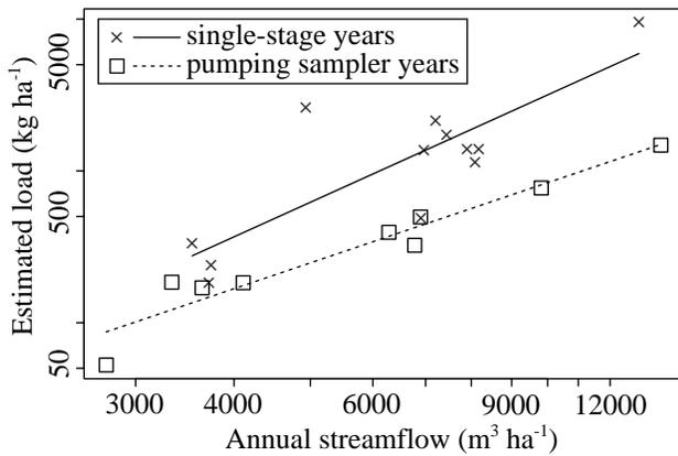
**Figure 5**—Relations between estimated annual suspended sediment loads and annual streamflow at North Fork Caspar Creek (NFC) prior to logging. Illustrates that load estimates based on sediment rating curves depend systematically on sampling protocols.
