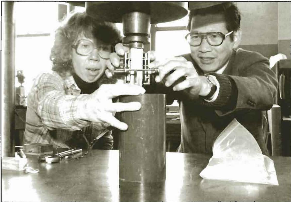
**Figure 1**—Training is critically needed in tropical institutes. At the USDA Forest Service's Forest Products Laboratory, a scientist from China learns how to use a universal testing machine from a Laboratory specialist.
