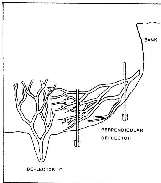
**Figure 2** — Cross section of the eroding bank showing deflector C and a set of perpendicular deflectors.
