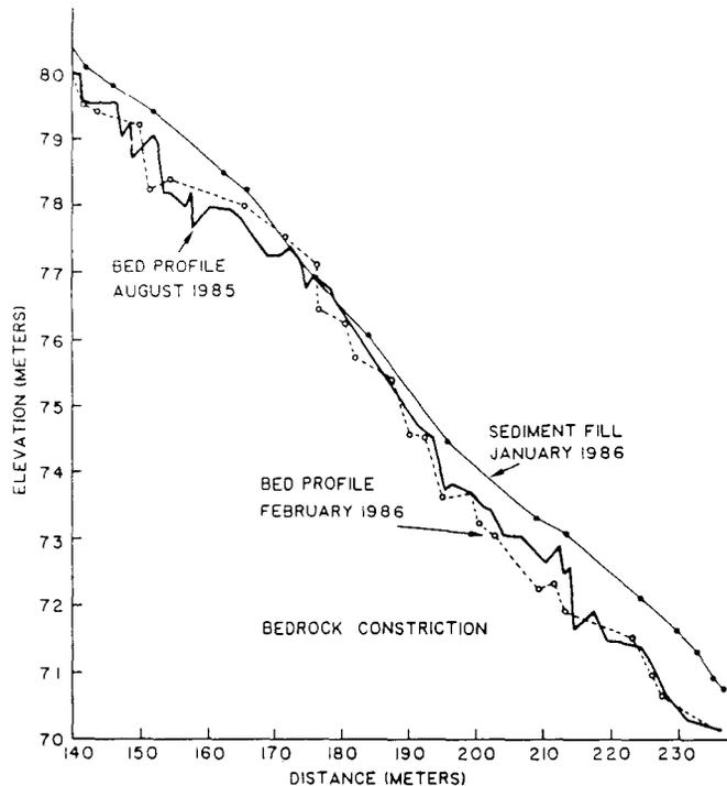
**Figure 3**— Longitudinal profile of lower portion of the study reach. Bed profile surveyed in August 1985; following the January 30-31, 1986 event; and following the February 13-15, 1986 event. Constriction extends from approximately 170-200 meters.
