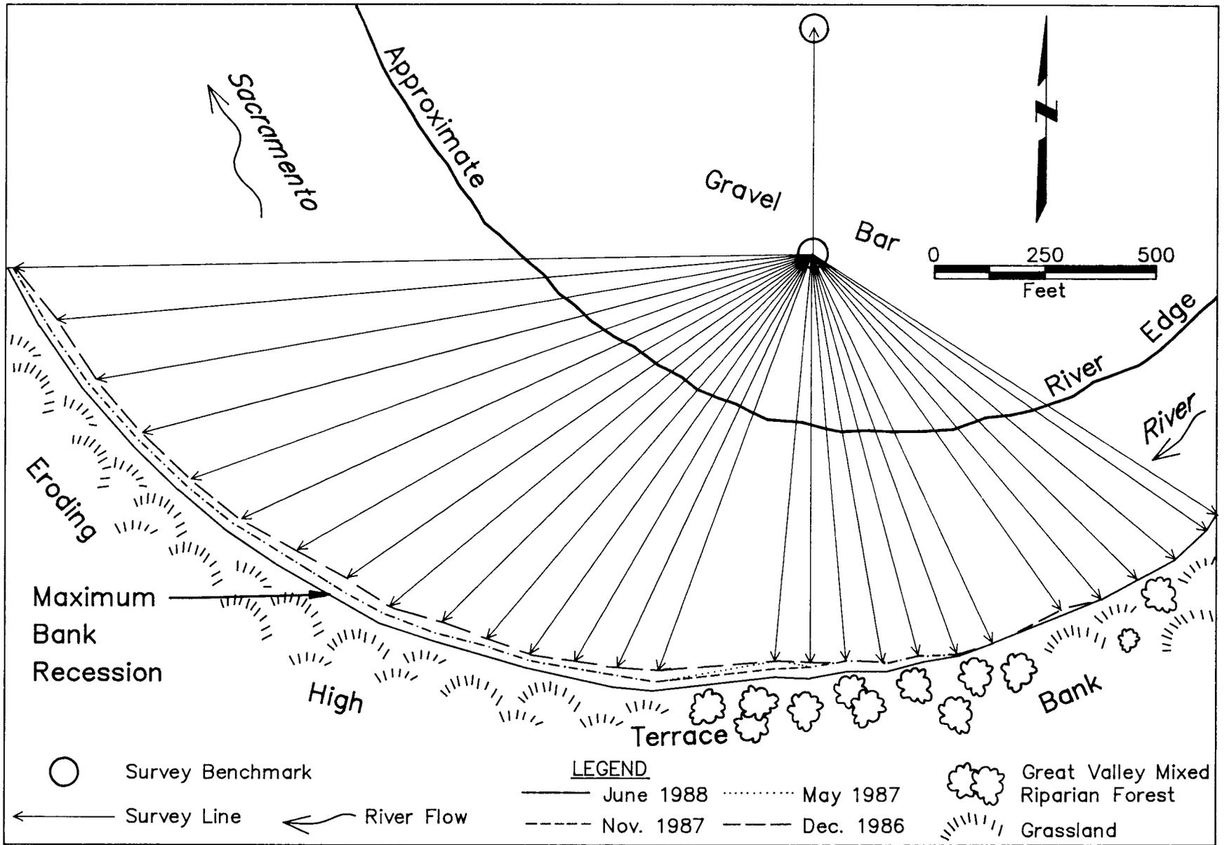
Figure 2— Golden State Island Surveyed Erosion Site December 9, 1986 through June 7, 1988
