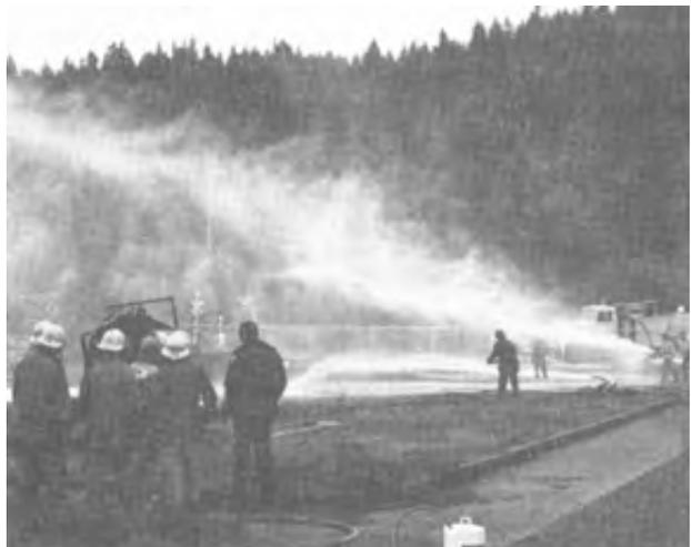
Figure 1--Fine-bubble mist is expelled during initial discharge from compressed air foam system.
