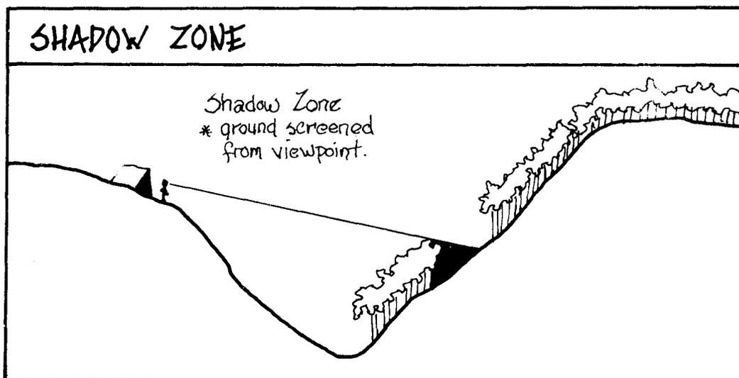
Figure 7--Shadow Zone is the amount of ground screened from view by foreground vegetation.
