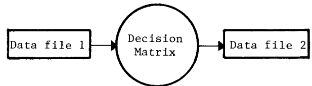
Figure 1--The "transform" option of VMSS allows data (File 1) to be simply relabeled or sorted into groups as specified by the decision matrix. File 2 is the resulting output of the transform process.
