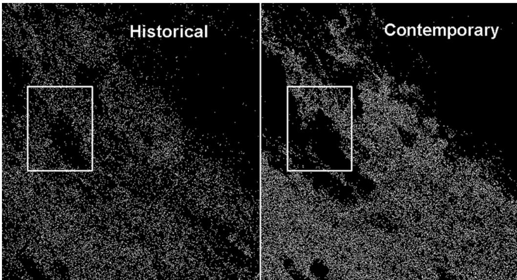
FIGURE 3. Comparison of locations of tall-stature woody vegetation (individual trees) using contemporary LiDAR remote sensing (2008) and historical aerial photography (1954). The data are shown as binary values, where white indicates tree presence, and black indicates tree absence. The box indicates areas of confirmed reduction in woody vegetation cover.
