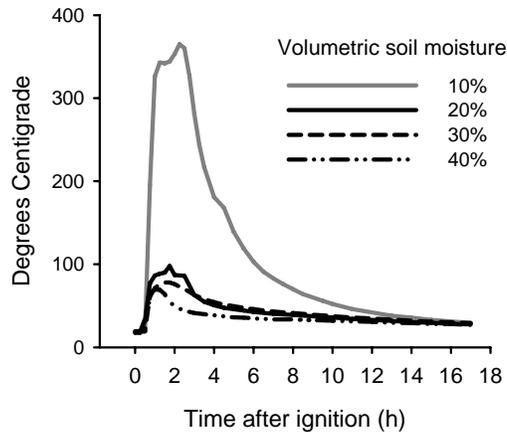
Figure 1. Effect of soil moisture on maximum soil temperature. Response curves are for the pumice soil at a soil depth of 1 inch and a masticated fuel load of 60 tons/acre.
