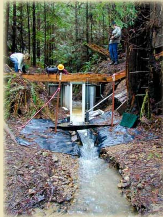
*Stream gage and sediment sampling station in a tributary of North Fork Caspar Creek.*
