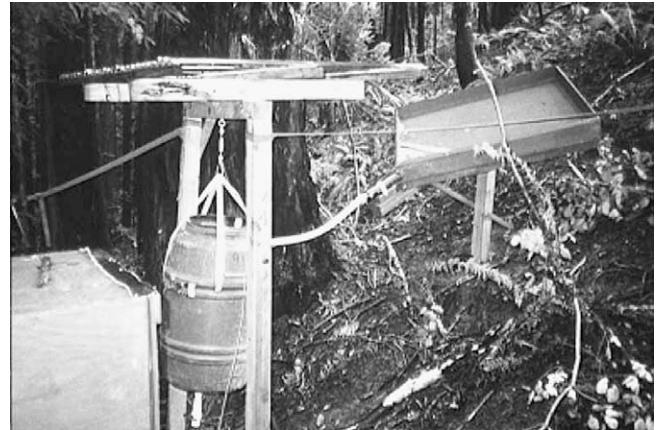
Fig. 1. Throughfall collector (1.2 m × 1.2 m) and plastic storage barrel, which is suspended from a load cell.
