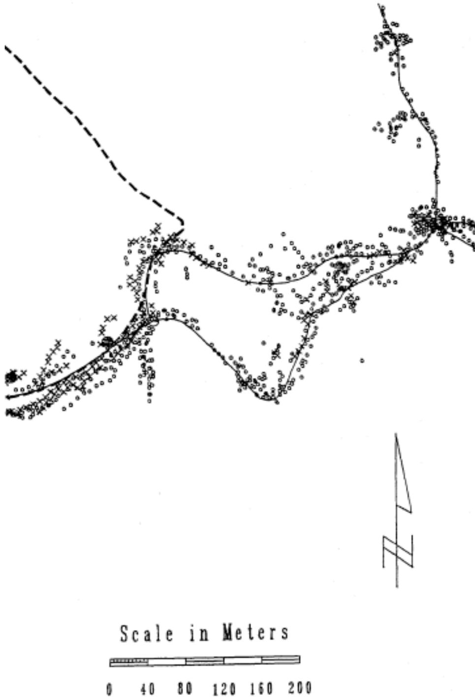
Figure 4. Map generated by computer and plotter from GPS data. Original map uses color to indicate differences between corrected and uncorrected points.
