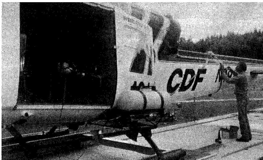
*Figure 2. Mounting the GPS antenna on the helicopter.*
